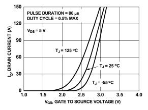
Figure 5. Transfer Characteristics
