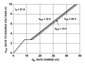
Figure 7. Gate Charge Characteristics
