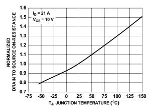
Figure 3. Normalized On-Resistance vs Junction Temperature
