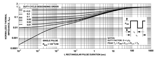
Figure 13. Junction-to-Ambient Transient Thermal Response Curve
