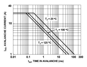
Figure 9. Unclamped Inductive Switching Capability
