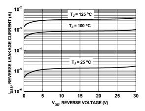
Figure 15. SyncFET body diode reverses leakage versus drain-source voltage
