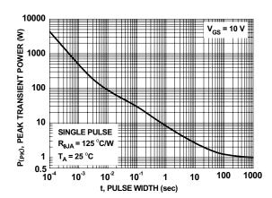
Figure 12. Single Pulse Maximum Power Dissipation
