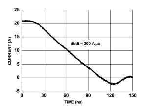
Figure 14. FDMS7670AS SyncFET body diode reverse recovery characteristic
