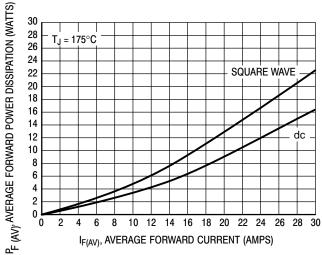
Figure 6. Forward Power Dissipation
