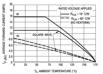
Figure 5. Current Derating, Ambient Per Leg
