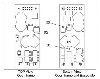
(Best air flow direction is from negative to positive pins.)
