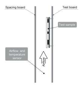
For products with base plate used in a sealed box/cold wall application, cooling is achieved mainly by conduction through the cold wall. The Output Current Derating graphs are found in the output section for each model. The product is tested in a sealed box test set up with ambient temperatures 85, 55 and 25°C.
