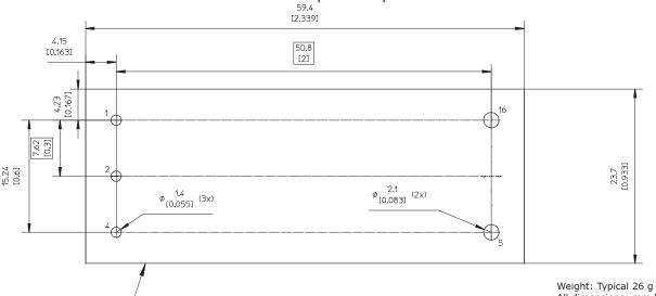
Recommended keep away area for user components. The stand-off in combination with insulating material ensures that requirements as per IEC/EN/UL60950 are met and 2250 V isolation maintained even if open vias or traces are present under the DC/DC converter.
