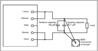
Output ripple and noise test setup
