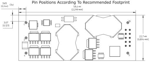
PIN SPECIFICATIONS Pin 1-5 Material: Copper alloy Plating: Min Au 0.1 µm over 1-3 µm Ni. Pin 5 Material: Brass Plating: Min Au 0.2 µm over 1-3 µm Ni.
