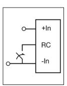
voltage generated on the RC pin is max 6 V. The standard product is provided with "negative logic" remote control and will be off until the RC pin is connected to the -In. To turn on the product the voltage between RC pin and -In should be less than 1 V. To turn off the product the RC pin should be left open for a minimum of time 150 us, the same time requirement applies when the product shall turn on. In situations where it is desired to have the product to power up
