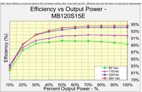
Note: Above efficiency curves are typical at 25C convection cooling, after 1 hour warm up time. Efficiency may vary with lower run time prior to measurement.
