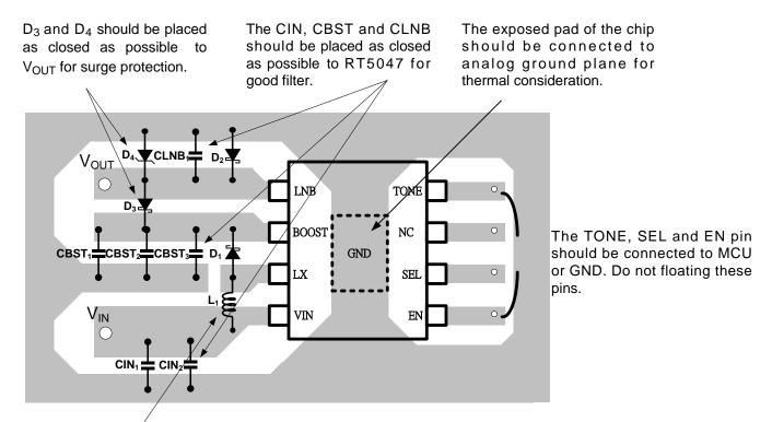
The inductor should be placed as close as possible to the LX pin to minimize the noise coupling into other circuits.
