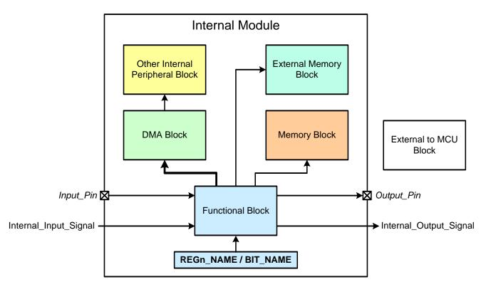
Figure 1.1. Block Diagram Conventions
