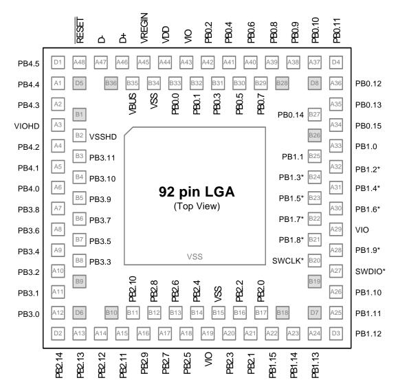
\*Noted pins are listed in the pinout table and 80-pin TQFP package figure with additional names. These alternate functions are also present on the 92-pin LGA package and are identical to those on the 80-pin TQFP package.
