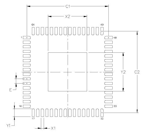
Figure 6.11. QFN-64 Landing Diagram
