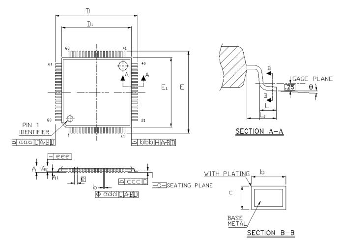
Figure 6.8. TQFP-80 Package Drawing
