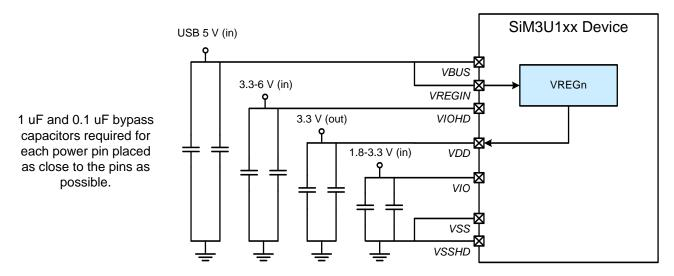
Figure 2.5. Connection Diagram with Voltage Regulator Used, USB Connected (Bus-Powered), and I/O Powered Separately
