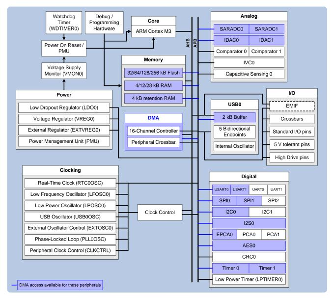
Figure 4.1. Precision32<sup>™</sup> SiM3U1xx Family Block Diagram
