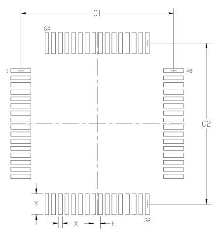
Figure 6.13. TQFP-64 Landing Diagram
