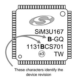
Figure 7.2. TQFP-80 SiM3U1x7 Revision Information
