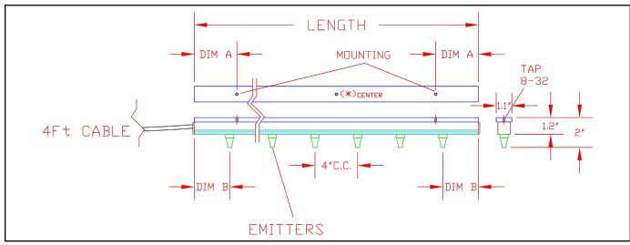
Figure 3. EMIT Non-Air Assisted Ion Bar dimensions
