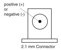
The board has a voltage regulator providing +3.3V and 1.8V. The regulator allows the input voltage to range from 7V to 9V. When you switch the power on, the red LED D11 marked PWR lights up. If it does not, switch off and check the power supply connections.
