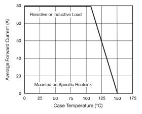
Fig. 1 - Forward Current Derating Curve
