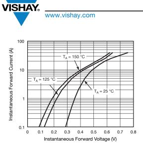
Fig. 3 - Typical Instantaneous Forward Characteristics Per Diode
