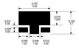
FIGURE 1. Recommended Copper Spreading Footprint
