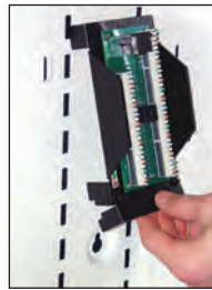
Step 1 - Mount on grid
