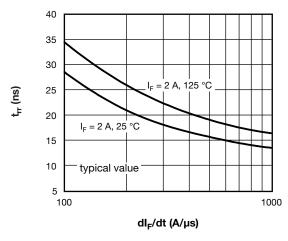
Fig. 6 - Typical Reverse Recovery vs. dl<sub>F</sub>/dt
