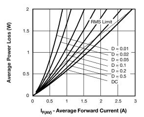
Fig. 5 - Forward Power Loss Characteristics
