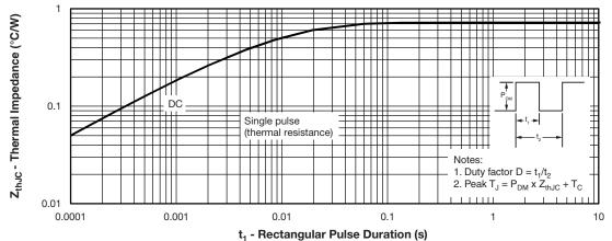
Fig. 4 - Maximum Thermal Impedance Z<sub>thJC</sub> Characteristics (Per Leg)
