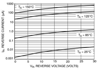
Figure 3. Leakage Current
